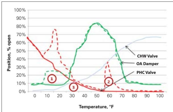
Figure 14: Using Pathian Curves for Ongoing Commissioning and Fault Detection
