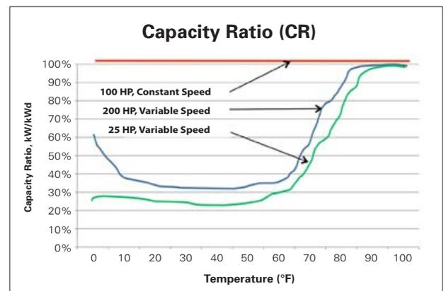
Figure 15: Capacity ratio for supply fans
