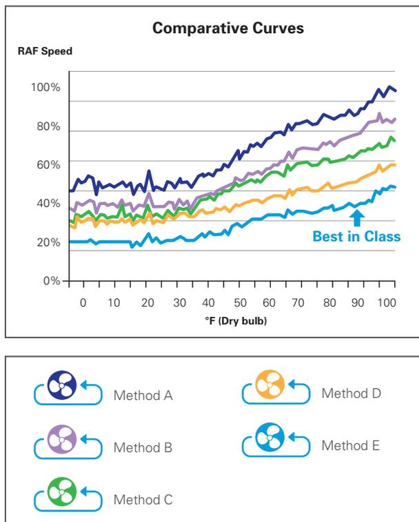
Figure 18: Control Sequence Benchmarking for different return fan control strategies
