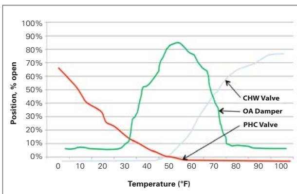
Figure 16: Position Benchmarking Curves for valves and dampers
