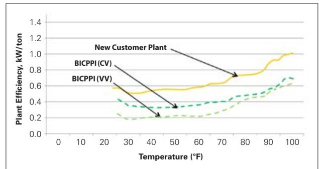
Figure 13: Using BICPPI curves for automated energy auditing
