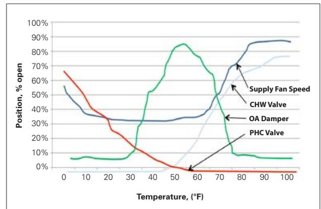
Figure 17: Load-to-Position Benchmarking curves for fans, valves and dampers
